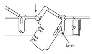
Figure 4. Loading the keystone jack or support fitting.
